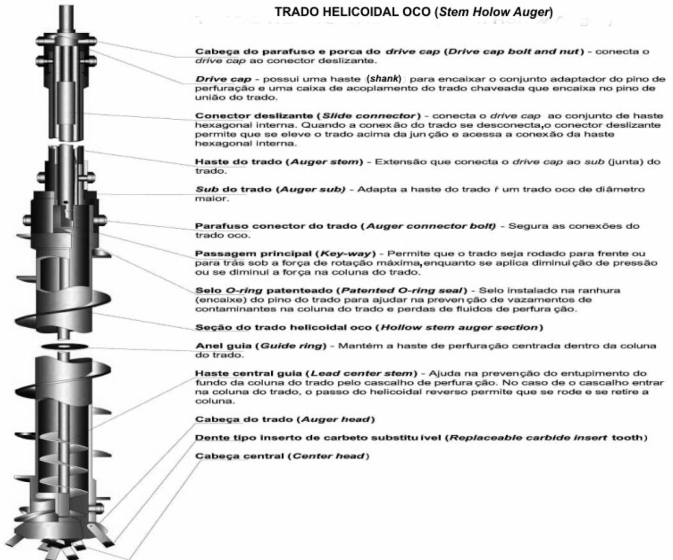
Figura 2 — Trado helicoidal oco (*Hollow stem auger*)
